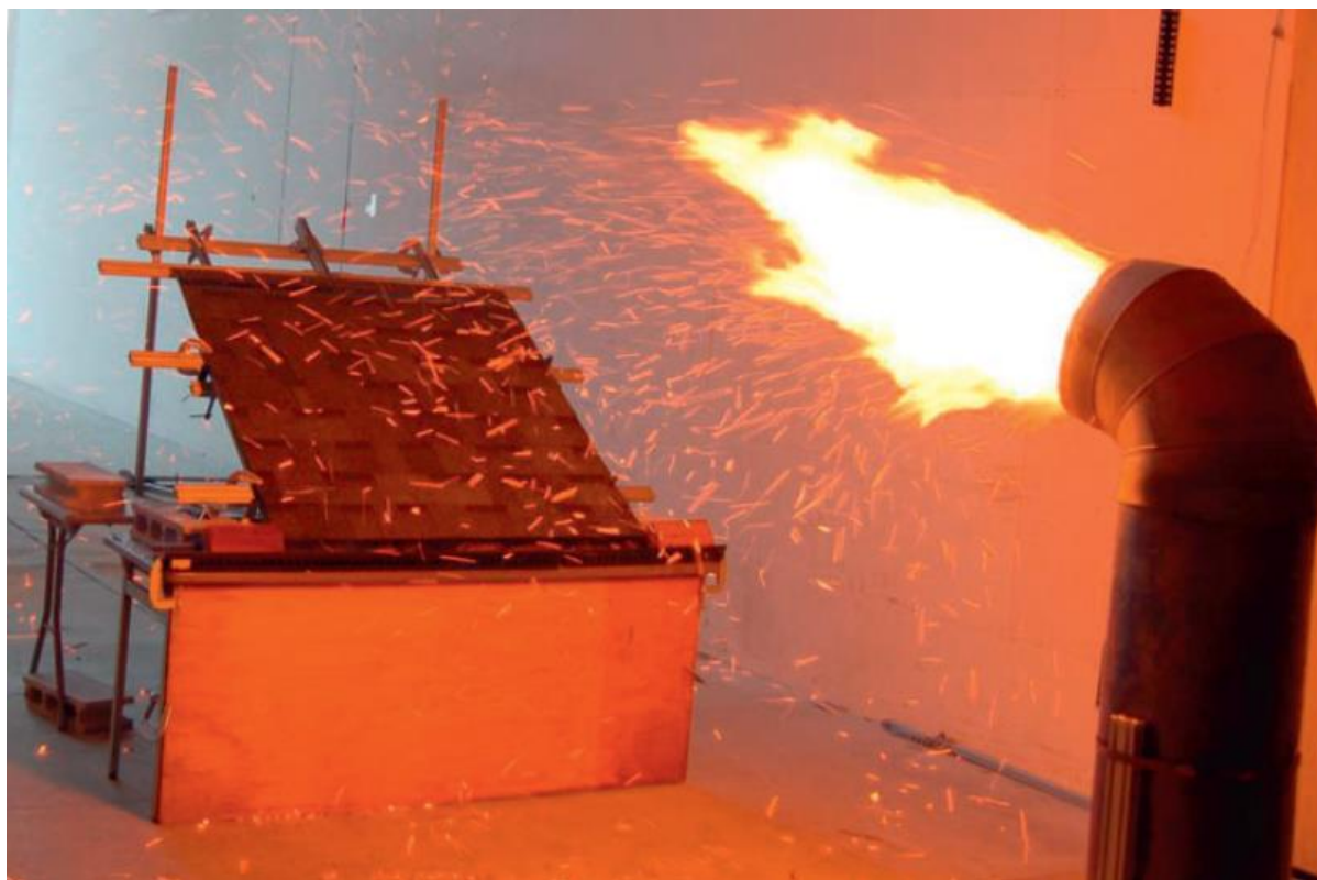
Figure 1. NIST firebrand generator testing exposure of a roof to embers.
