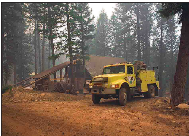
Figure 15. Turnaround adequate for fire pumper.
