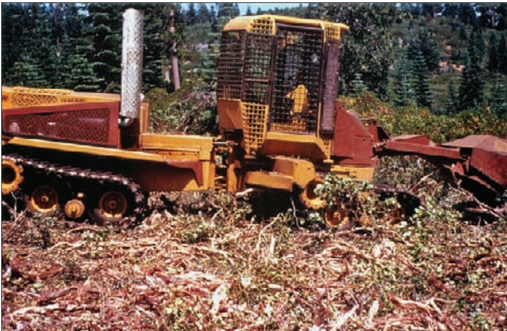
Figure 16—A Trac Mac at work in an older plantation. Note the layer of shredded vegetation in the foreground.
