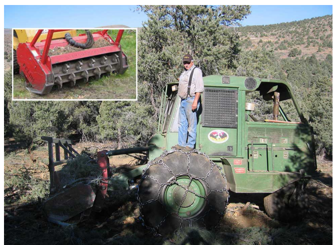
Mechanical mastication, such as with this single-operator machine, is one type of treatment for thinning plots of live, mature pinyon stands. Photo: USGS.
